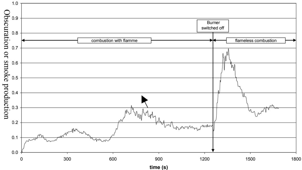
Figure 4: Smoke production of a cellulosic product (plywood) during flaming and non-flaming fire condition. Smoke production is highest after the ignition source has been switched off, during non-flaming or smouldering condition [10].
