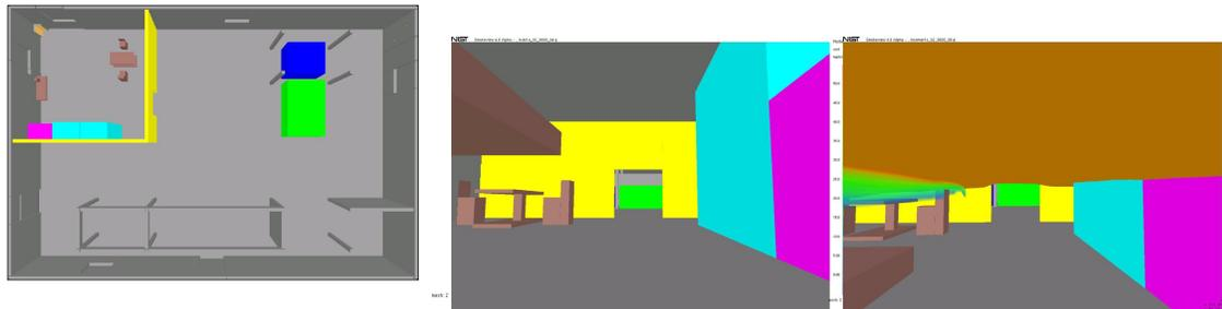
Figure 6: a. ground plan of industrial building with office, fire sources indicated, b. situation before ignition, view from the office facing the doorway, c. smoke layer after 600 s, boundary layer with soot mass concentration of  $24 \text{ mg/m}^3$ , extinction-coefficient:  $0.27 \text{ m}^{-1}$ , visibility: 30 m [10]
