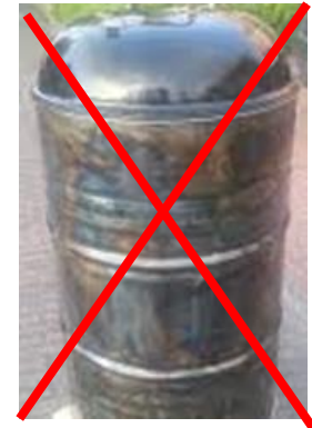
Drum too quickly closed after decontamination
