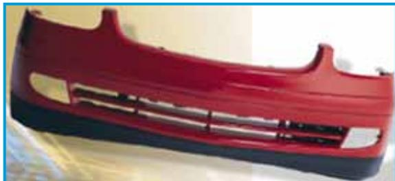
The excellent shock absorption properties of polyurethane in, for example, bumpers and dashboards ensure the safety of drivers, passengers and pedestrians.
