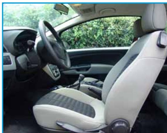
In the last five years the density of polyurethane for major applications has been reduced by 30 to 40 per cent while still maintaining the same mechanical properties. Seating foam, for instance, has one of the lowest densities of any plastic material used in a car: 0.03 to 0.05 g/cm<sup>3</sup>. Polyurethane foam in headliners is another good example with a density of 0.02 to 0.04 g/cm<sup>3</sup>.
