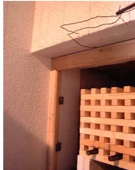
Fig. 4 – Wooden crib for fire exposure
