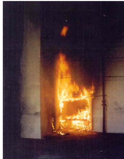
Fig. 7 – Fire after 14 minutes with burning window frame and burning rolling shutter box
